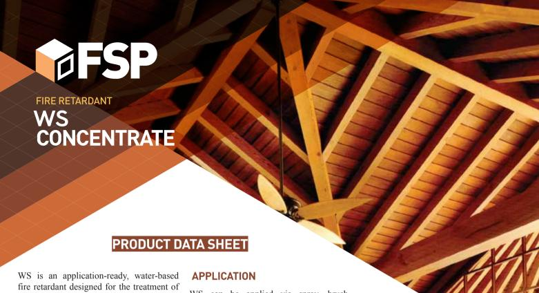
WS is an application-ready, water-based fire retardant designed for the treatment of raw wood. It is a mix of proprietary ingredients that forms a slight intumescent foam layer and carbon char when the treated wood is exposed to fire. Once the carbon char is formed, there will be minimal flame propagation, smoke evolution, or afterglow. The product is designed for interior applications and may be used on exterior applications with a approved top coat.
